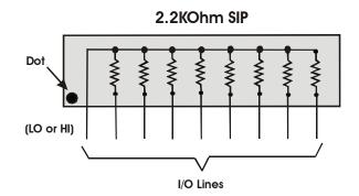
Figure 4-1. Eight-resistor SIP schematic
